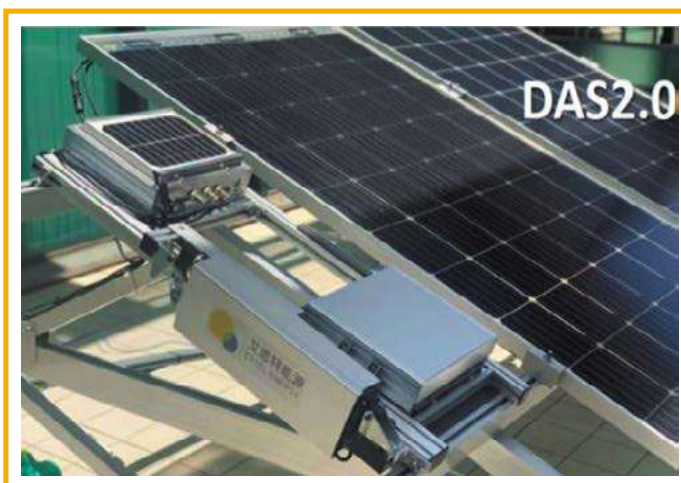
▲Photo: Dust monitoring system to assist in optimizing module cleaning frequency
